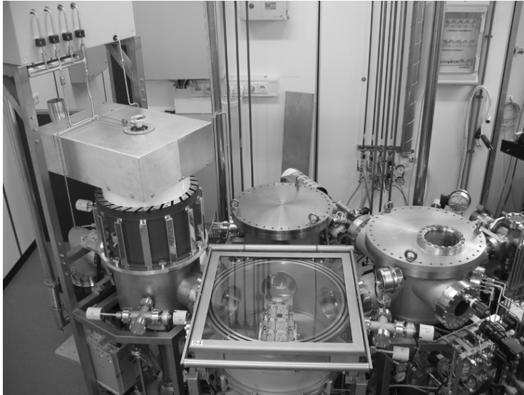
Figure 3.3: photograph of the loadlock (front) with three ALD systems, from left to right: 1. low temperature plasma enhanced deposition of dielectrics, 2. deposition of TiN layers and 3. deposition of Al 2 O 3 dielectrics with in-situ RHEED system.
